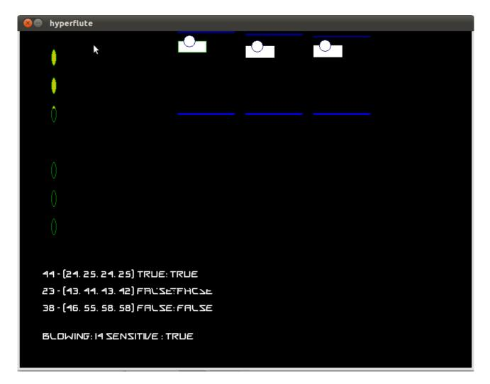
When the software has identified a note from the recorder it plays it on either a square or saw-tooth wave using the Minim library.
