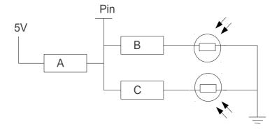
Because resistances B and C are different, the overall resistance of the sub-circuit will also change depending on which LDRs are occluded. With sensible choices of A, B and C and software calibration, the four possibilities (neither, B, C, both) can be distinguished. With this method, 4 analogue input pins can accommodate the 8 holes and still have one left for the breath input.
