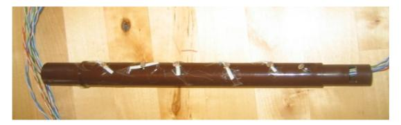
The LDR was just small enough to slip through so I needed to find a (reversible) way to hold it more or less at the position of the hole. I eventually settled on the idea of using a short piece of plastic "tag" threaded between the two legs of the LDR, and then taped across the hole. The plastic tag therefore separated the two legs of the LDR, (ensuring they didn't short) and prevented the LDR sliding inside the body of the recorder.
